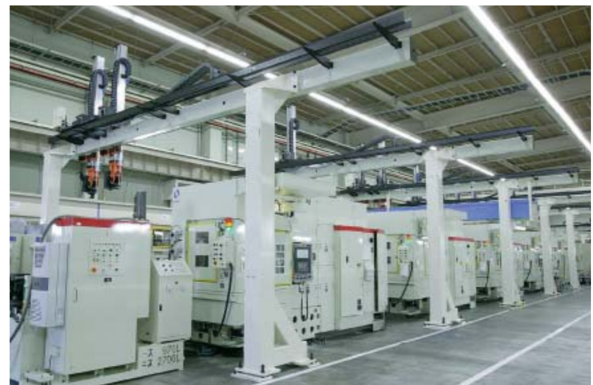
Automatic transfer (gantry loader)
