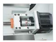
Three axes equipped with precision ball screws class C3 and diameter 40 mm pitch 16mm
