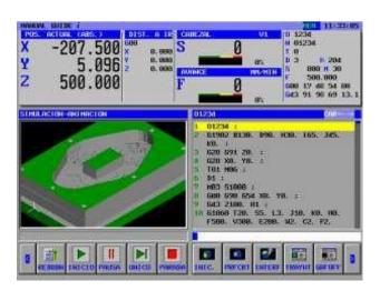
The conversational Manual Guide i system allows programming in ISO function, or by Fanuc canned cycles, as well as combining the two, which greatly facilitates operations.
