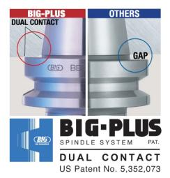
The BBT40 double-contact taper main spindle interface is fitted as standard. This improves the machining performance of the machine by eliminating vibrations caused by the gap between the tool holder and the spindle nose.
