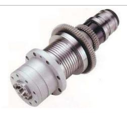
High-quality machining guaranteed by incorporating high precision bearings, class P4. The tool anchoring system is floating. This ensures a good clamping of the tool to the spindle without transmitting stress to the bearings of the spindle and ensures longer life to the bearings. The spindle is cartridge type.
